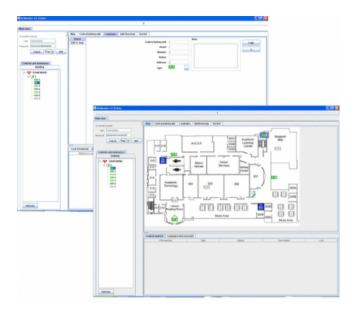
Web Advanced Central Monitoring software (WebACM) is a centralized remote monitoring system, which connects to an Ethernet network, for our addressable central battery systems.
